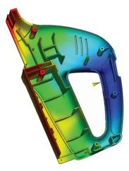
**Packing** Optimize packing profiles and visualize magnitude and distribution of volumetric shrinkage to help minimize plastic part warpage
