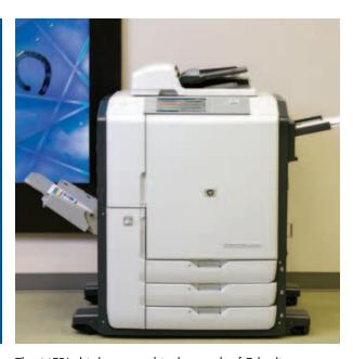
The MFP's higher speed is the result of Edgeline Technology hardware innovations. It utilizes printhead arrays that are the full width of the page. Rather than moving a narrow printhead back and forth across the paper (like most inkjet printers), the paper passes beneath the printheads. Paper can move continuously beneath the printheads at speeds of up to 35 inches per second.
