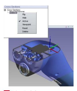
**Derive 3D Cross-Sectioning** Create section views of mechanical or machine designs to understand how the parts are assembled.
