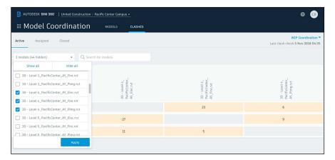
PRO TIP: Search and filter models within the clash matrix (using model naming conventions) to focus review on a specific location. Click on the row header to open and view all models and clashes within that context.
