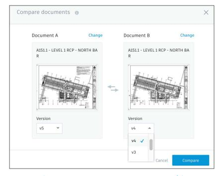
PRO TIP: With 2D compare, you can compare two versions of the same drawing or model or two entirely different drawings. For example, you could compare drawings from two different disciplines.
