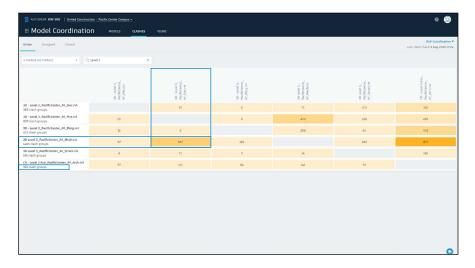
PRO TIP: By default you're taken to the Active sub-tab, which displays a grid of all the clashes that have not yet been reviewed. The Assigned sub-tab displays a list of clashes that have been marked as an issue, and allows you to track the changes being made to resolve the clash. The Closed sub-tab displays a list of clashes that have been marked as 'Not an issue.'
