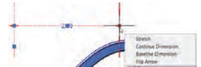
**TIP** Multifunctional grips are even more powerful when dynamic input is on. Use the Tab key to jump between input boxes.
