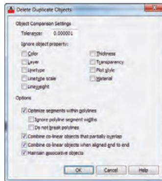
Control OVERKILL settings in the dialog box. Specify which object properties to ignore along with whether or not to optimize polyline segments and/or combine co-linear objects. The tolerance value controls the precision by which OVERKILL will operate.
