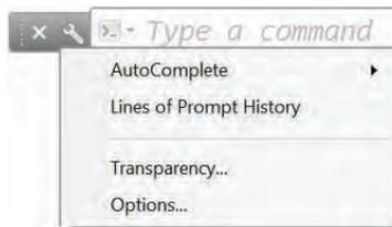
F2 (or the flyout at the right end of the floating command line) will display the history window. Click on the >\_ at the left to quickly access previously used commands.
