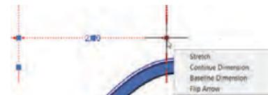
**TIP** Multifunctional grips are even more powerful when dynamic input is on. Use the Tab key to jump between input boxes.
