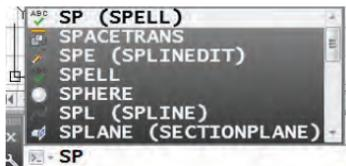
**TIP** Customize AutoComplete from the command line right click menu (even control the delay response time).
