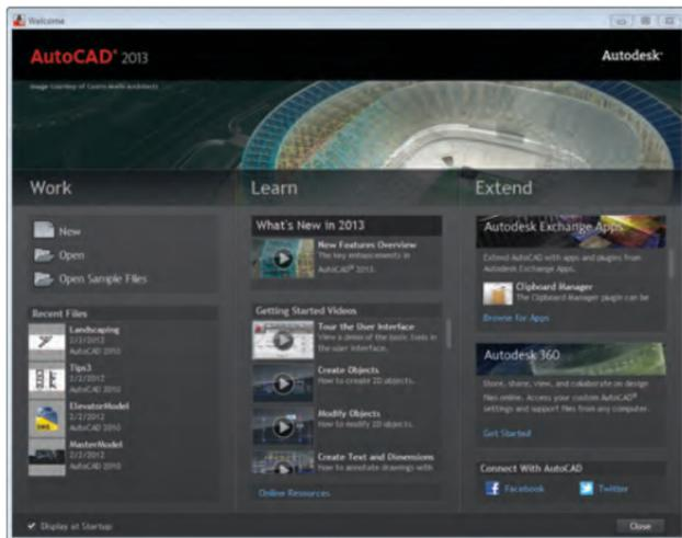
Create new or open existing drawings from the Work panel. You can also quickly access recently used drawing files.
