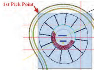
**NOTE** By default, SNAPMODE now temporarily turns off when selecting objects. This can be set back to legacy behavior in the SNAP command.
