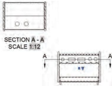
Use the Edit Components tool to modify the objects used in the Section View. If a component is set to none, it will not be sectioned.
