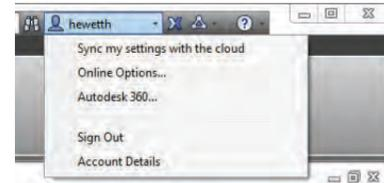
**NOTE** When you upload drawings from AutoCAD to Autodesk 360, external references and other dependent files upload as well!
