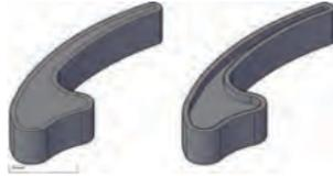
Follow this up with Presspull or Extrude to easily add or remove the bounded area from a solid.
