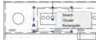
Easily modify a detail view after the fact by using grips on the detail symbol, view or view label or on the Detail View
