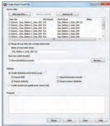
Indexing provides a noticeably smoother and faster workflow. The new Create Point Cloud File dialog allows you to select multiple files to batch index and even merge into a single file.
