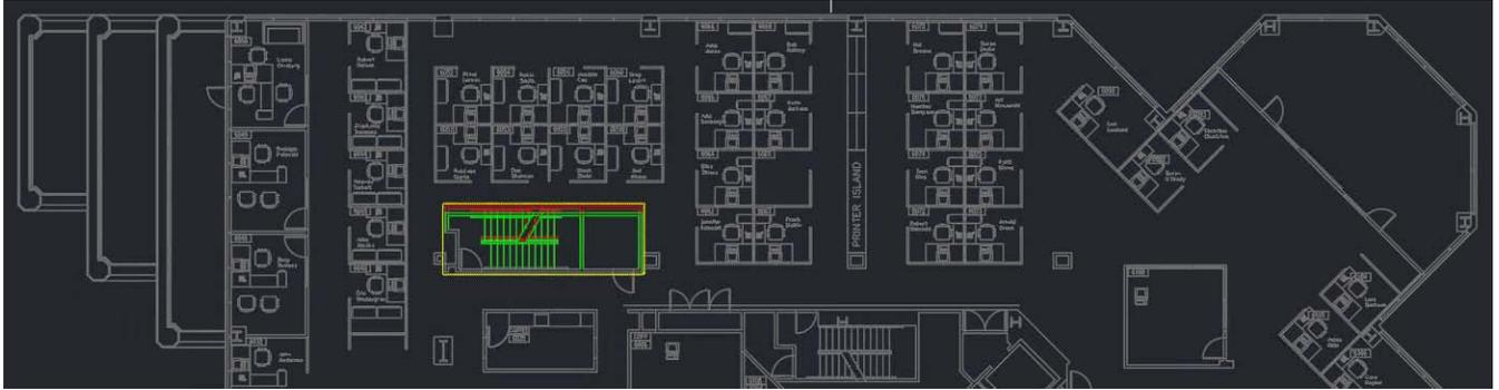
The green and red graphics highlight the differences between the first version of the drawing (green) and the second version (red). All unchanged elements are shown in grey. Having displayed this important difference, now you can adjust the positions of the cubicles adjacent to this exit stair to maintain the required clearance.
