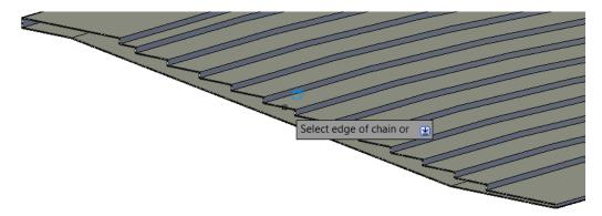
The Chain option within the FILLETEDGE command identifies and fillets edges that have continuity. For example, the part below on the left does not have rounded corners so the fillet operation is limited to the selected edge. The part on the right, however, has rounded corners enabling the Chain option to select and fillet all the continuous edges.
