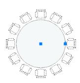
If you want to change the appearance of all the arrayed objects, there's no need to start over. You can edit the source object in place. AutoCAD automatically displays the Edit Array contextual tab in addition to the many AutoCAD drawing and editing tools. After making edits to the source geometry, or if you decide against editing the geometry, you can choose to save or discard changes.
