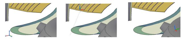
You can rotate the UCS around the X, Y, or Z axis using grips, and without having to access the UCS command.
