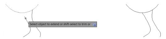
The 3D Edit Bar is enhanced to support splines and is accessible from the right-click menu when a spline is selected. It enables you to move the location of a point on the curve, change the magnitude of the tangency at the point, and change the tangent direction relative to the point.
