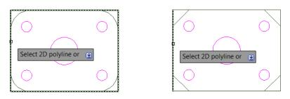
If the preview is not as desired, you can edit the fillet radius or chamfer distance/angle prior to completing the operation.
