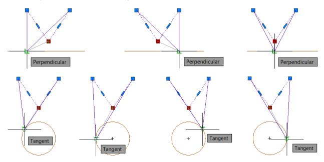
If Infer Constraints is enabled when using the perpendicular or tangent object snaps, the corresponding geometric constraint is automatically applied to the objects.
