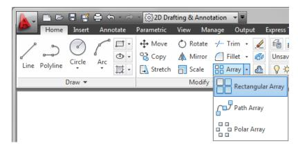
Using the new array functionality you can establish and maintain a set of relationships between arrayed objects. As you create the array, AutoCAD displays a preview with grips that you can use to visually edit array properties. Even after creating the array, you can use the Properties palette or multifunctional grips to modify it.
