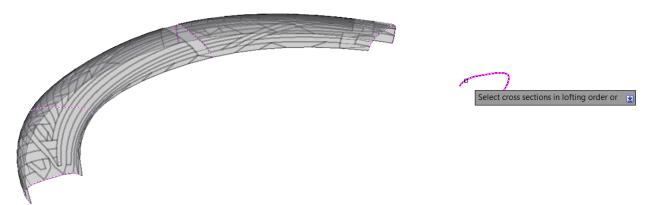
In addition to solid and surface lofts, the preview is included with the following commands: SURFBLEND, SURFPATCH, SURFFILLET, FILLETEDGE, CHAMFEREDGE, and LOFT. The preview displays with a transparency to easily distinguish it from completed objects. You can control the transparency level with the new PREVIEWCREATIONTRANSPARENCY variable.
