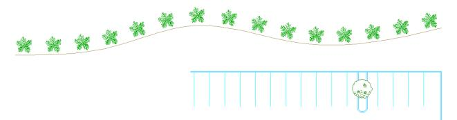
You can control the position of the arrayed items relative to the path using the Base Point option. Whether the base point of the arrayed object is on the path or offset, the items are associated with the path. When the path changes, the items automatically update.
