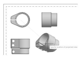
Each view creates a new Drawing View object, which includes a boundary similar to a viewport but does not print. An icon in the status bar tray indicates when a drawing contains drawing views, and you can view and modify properties for a selected drawing view using the Properties palette.
