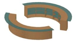
Whether you create one- or multiple levels of array objects, you can specify an increment value for row elevation. When the row elevation increment is set to zero, as it is by default, all rows are created at the same elevation. When set to any other value, positive or negative, the elevation of each row is incremented by that amount.
