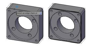
In addition to the Chain option, the FILLETEDGE and the CHAMFEREDGE command include a Loop option. A loop is similar to a closed chain. After selecting an edge, you can choose which of the potential loops to use.
