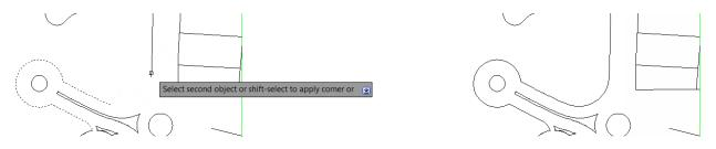
The new Blend tool creates spline objects with options for tangent or smooth continuity between two curves, speeding documentation time. It supports lines, arcs, 2D and 3D polylines, splines, helixes, and elliptical arcs.
