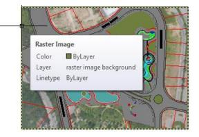
Similarly, passing the cursor over geometry inside an attached DWF, PDF, DGN, or DWG file displays a selection preview frame. You can select the frame for any of the attached reference files to display a frame boundary, with the ability to grip-edit a clipped boundary frame.
