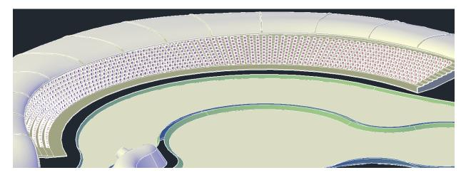
When creating a path array, you can specify whether the arrayed objects should maintain a vertical orientation (Z direction) or adjust to remain parallel to the path.
