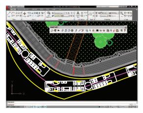
>> Create a vehicle path that maintains a minimum clearance from a roadway element (i.e. curb, barrier, paint line, pavement edge, etc).
