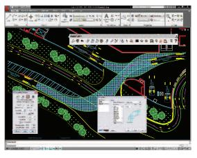
>> Powerful features make vehicle reverse maneuvers easier than ever. Hatch vehicle body envelopes and swept paths to check for clearances.
